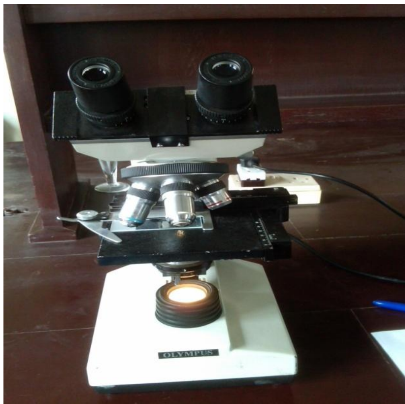
Plate 3.3: Picture of the Light Microscope used for morphological assessment of the Spirogyra filaments
