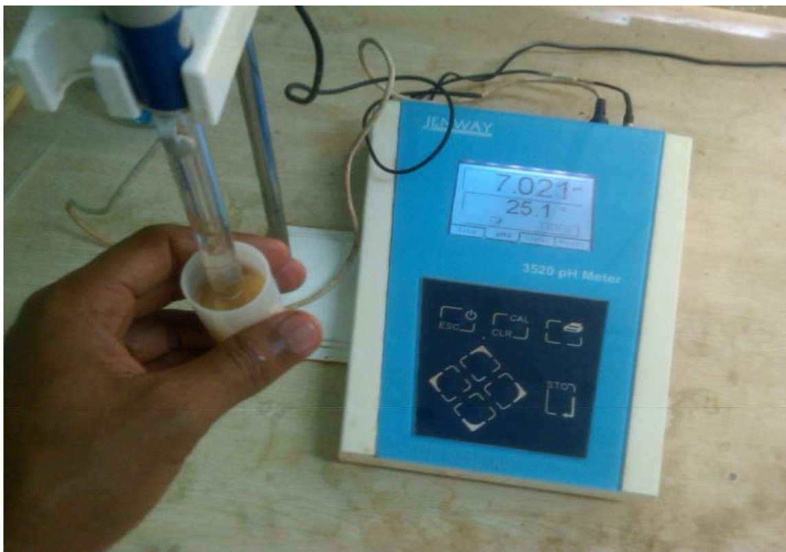
Plate 3.20: Showing the pH of one of the oils being determined using Jenway ® 3520 model pH meter
