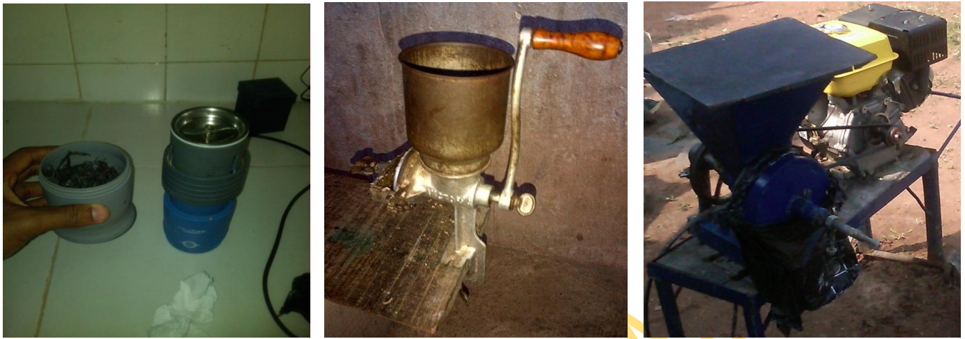
(a) (b) (c) Plate 3.8: Showing the instruments used for pulverization/milling-(a) Miller (IKA ® A11 BS2 model); (b) Hand-powered bench grinder (c) Fuel-powered domestic grinder
