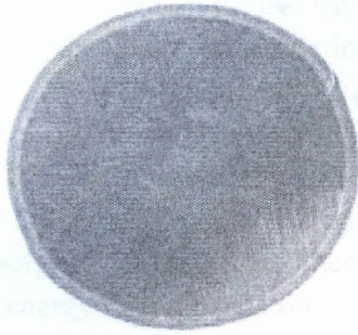
Plate 1(a) Macrostructure of a specimen, carburized at 940°C for 3 hours The carburizer contained 20% Na 2 CO 3 Etched in 25% Nital. Magnification : x 2
