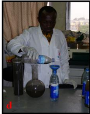
d. Supernatant was filtered with 2.5µm filter to remove suspended particles.
