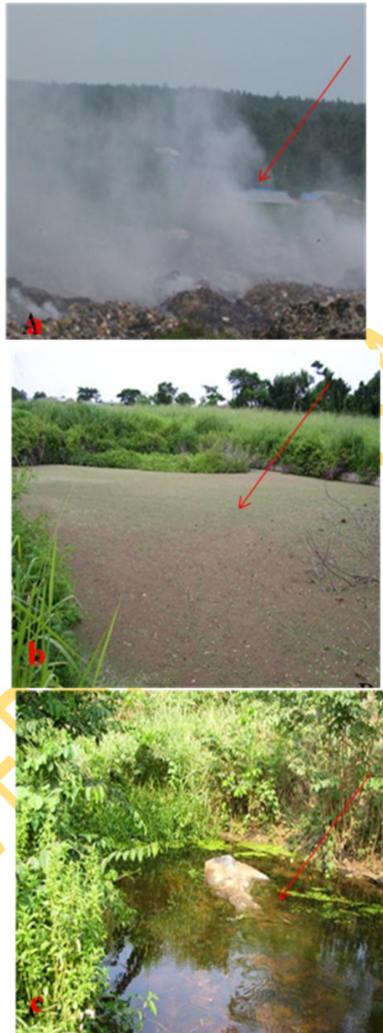
Fig. 3.3 (a) Burning and residential quarters (red arrow) within Aba-Eku landfill. (b) Leachate well (red arrow) meant to receive leachate from the dumpsite for subsequent treatment but no longer functional, hence discharges leachates into Omi stream.
