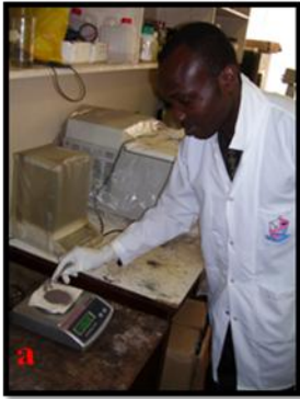
a. 250g solid waste soil sample was weighed into volumetric flask
