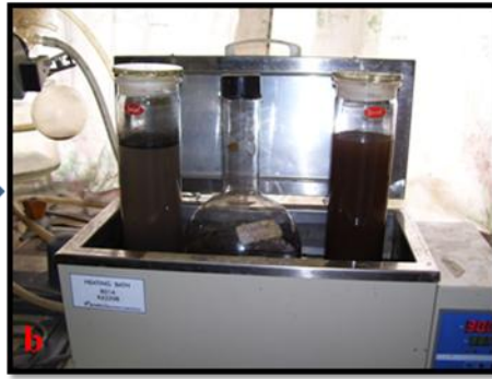
b. 1000ml of distilled water was added to form soil solution.
