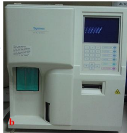
b. Automated analyser machine for use to quantify haematological indices.
