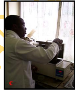
c. Soil solution was mechanically stirred at 1 hr interval using glass rod for 24 hrs
