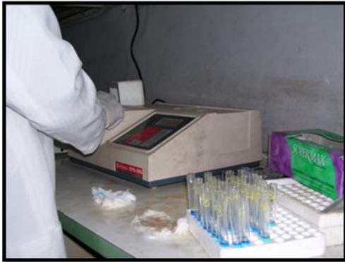
d. Absorbance of the biochemical parameters were read spectrophotometrically against blank.
