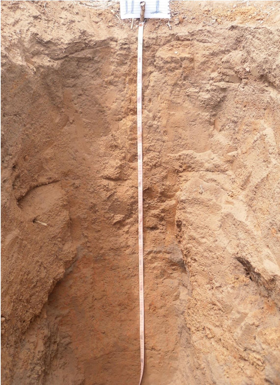
Plate 1: Iseyin series (Ferric luvisol) found at Ipapo with sandy clay to sandy clay loam subsoil and dark red hue down the profile.
