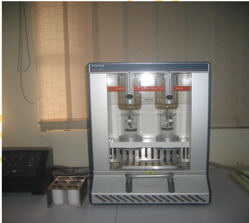
Plate 3.11: Digester Foss Tecator 8
