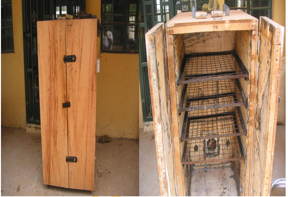
Plate 3.3: Close and Open Views of Fish Kiln Constructed for the Study
