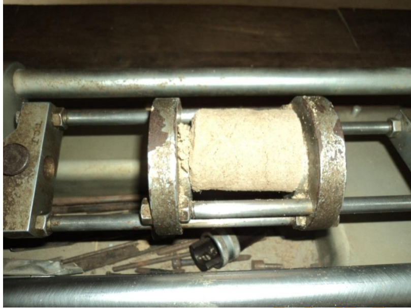
Plate 3.20: Briquette Failure under Compressive Load
