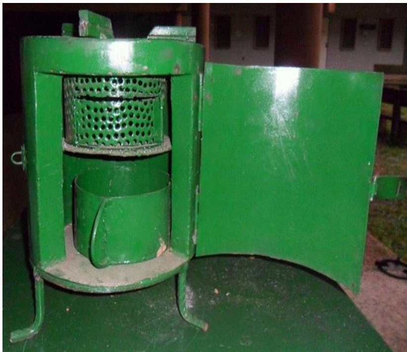
Plate 3.14: Briquette Stove Showing the Insulated Stove Wall
