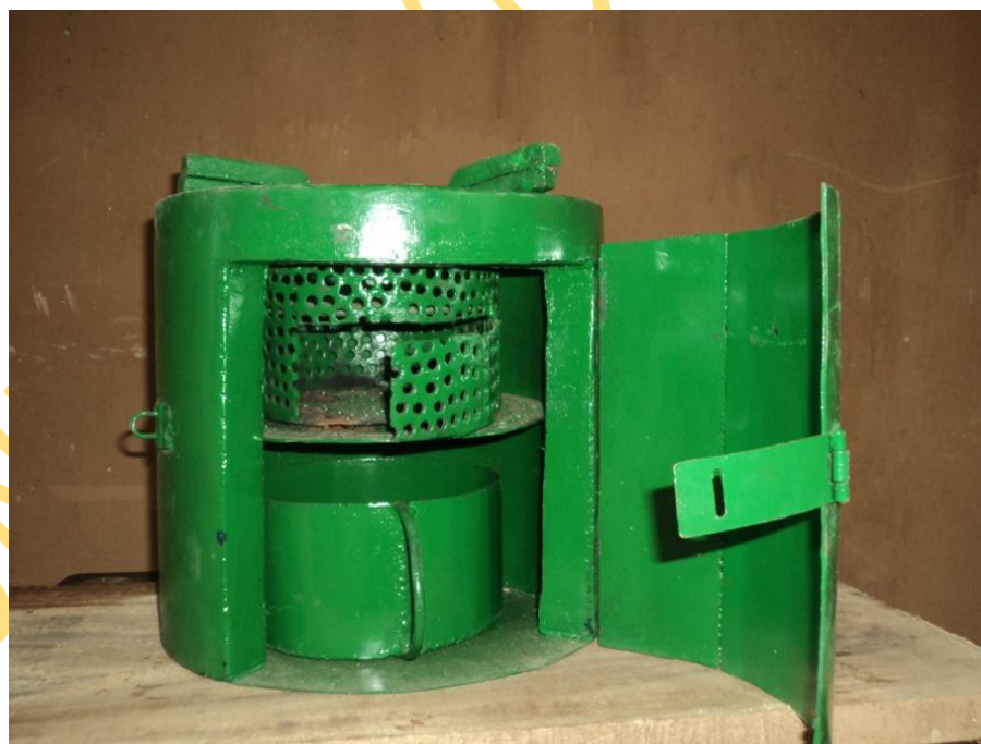
Plate 3.15: Briquette Stove with its Briquette Loading Door Wide Opened
