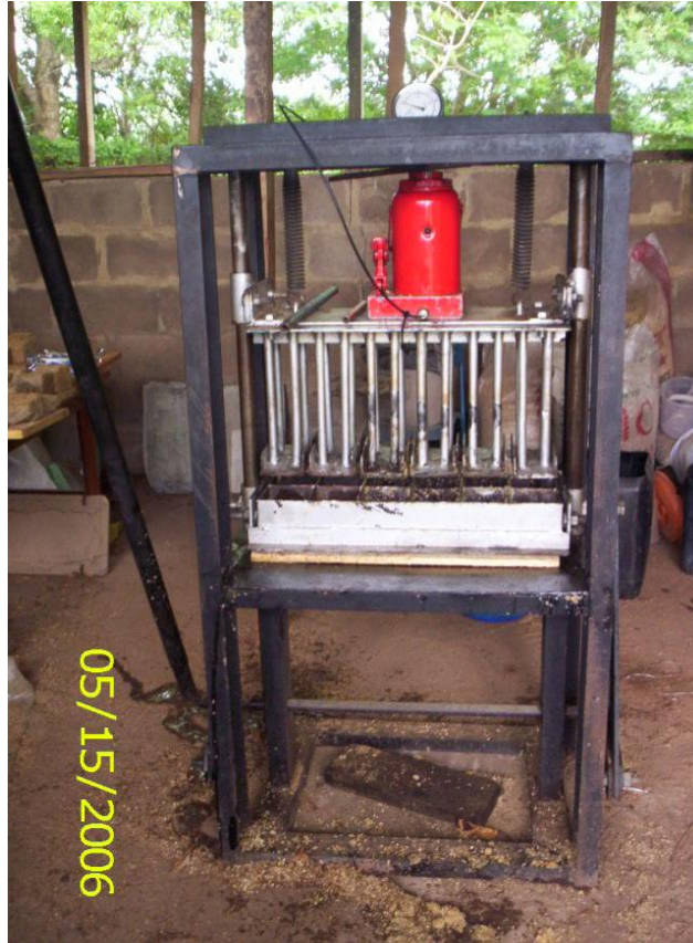
Plate 2.2: Manual Briquette Machine Produced by University of Ibadan Mission Research Team (Igbeka et al , 2005)
