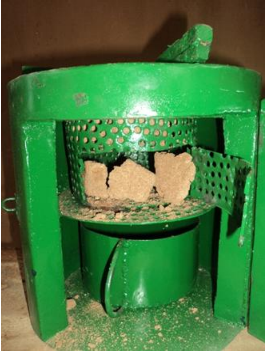
Plate 3.16: Briquette Burning Stove Loaded with Briquettes via the Loading Door
