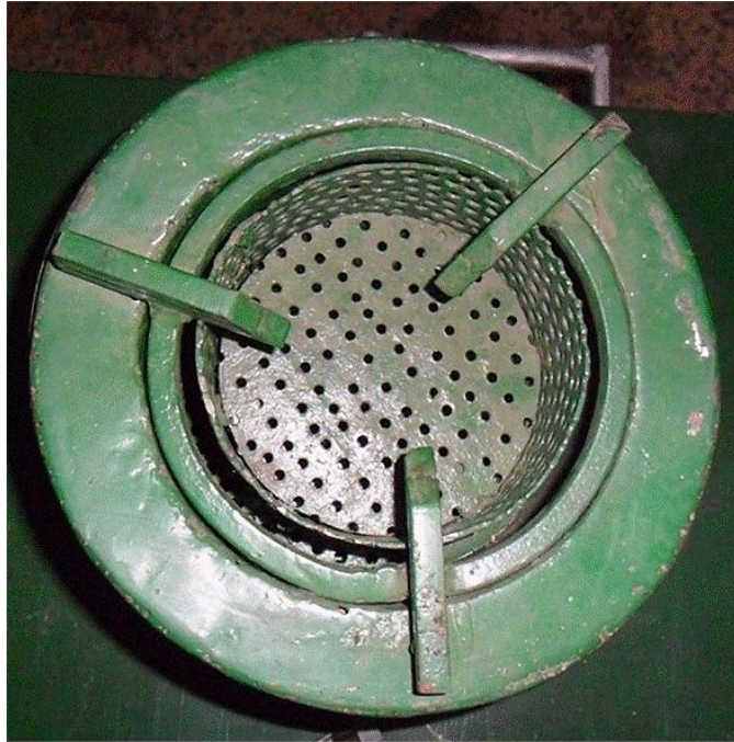
Plate 3.13: Vents on the walls and grates of the Combustion Chambers of Briquette Stove
