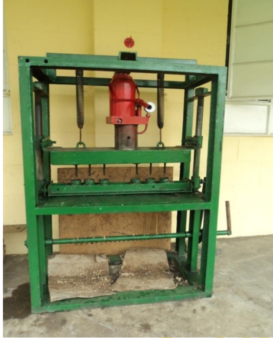
Plate 3.8: Modified Manual Briquetting Press
