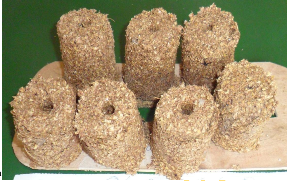
Plate 4.7: Samples of Maize Cob Briquettes produced from 1.18mm Particle Size, 25% W / W Binder Concentration at 1.5 MPa
