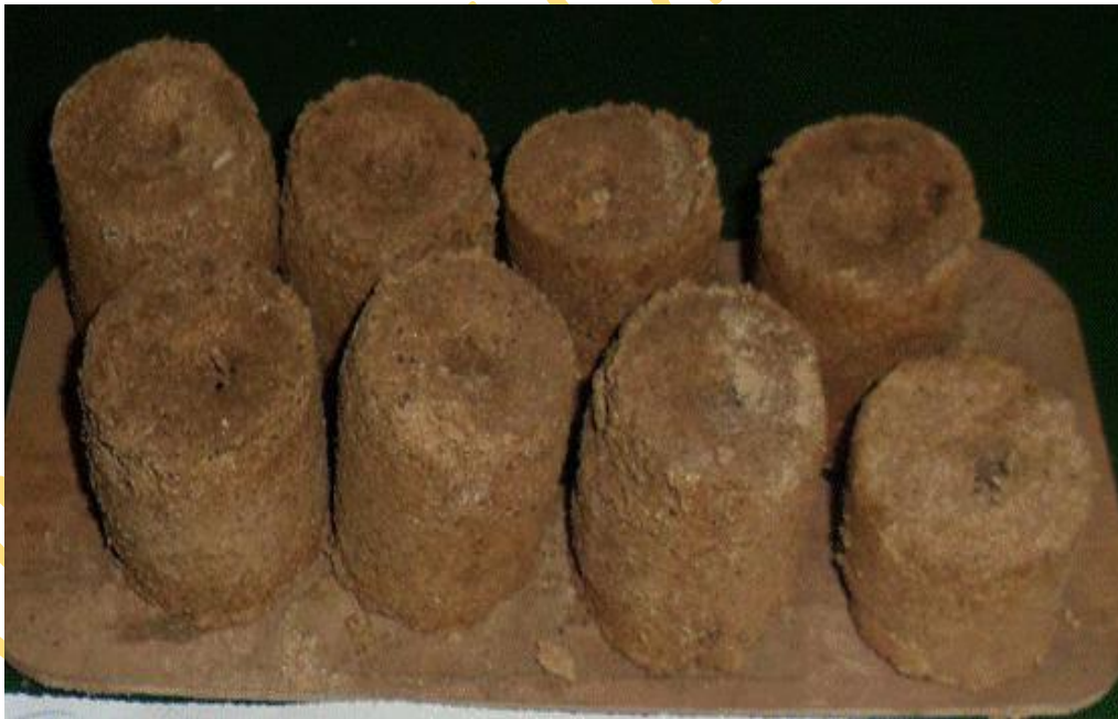
Plate 4.2: Samples of Sawdust Briquettes produced from 0.6mm Particle Size, 15% w/w Binder Concentration at 1.5 MPa
