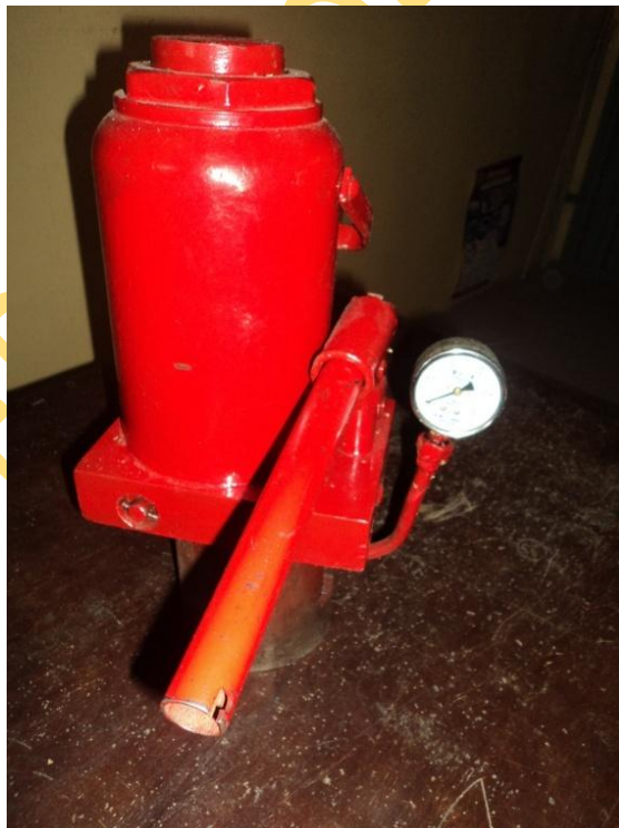
Plate 3.9: Hydraulic Jack (A Pressure Gauge was incorporated)
