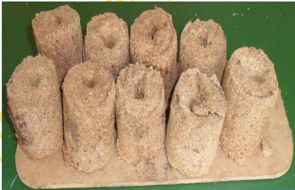
Plate 4.6: Samples of Sawdust Briquettes produced from 0.60mm Particle Size, 25% W / W Binder Concentration at 1.5 MPa
