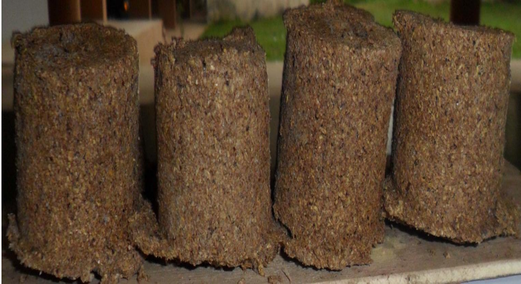
Plate 4.5: Samples of Maize Cob Briquettes produced from 0.60mm Particle Size, 25% W / W Binder Concentration at 1.5 MPa
