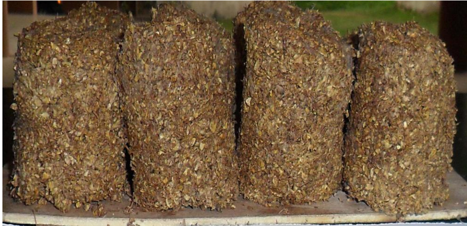
Plate 4.3: Samples of Maize Cob Briquettes produced from 1.18mm Particle Size, 20% W / W Binder Concentration at 1.5 MPa
