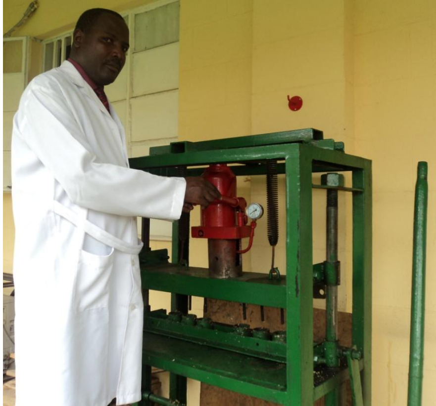
Plate 3.17: Compression of Briquettes with Manual Briquetting Machine
