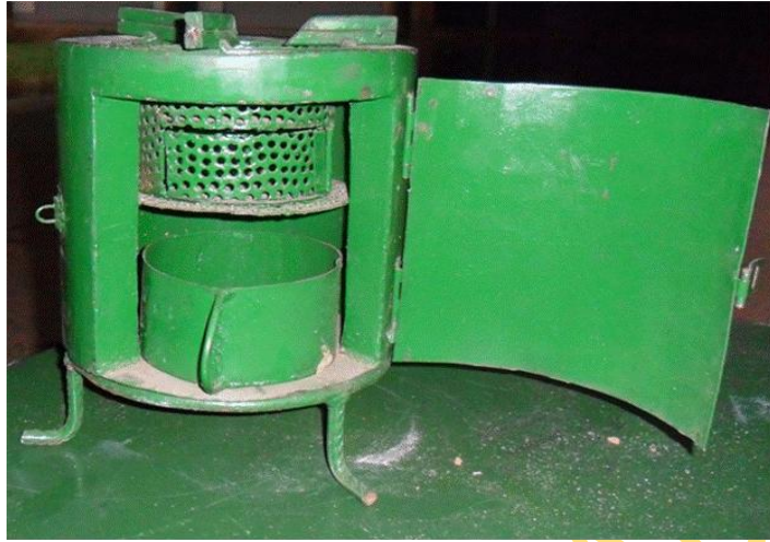
Plate 3.12: Ash Pit of the Briquette Stove
