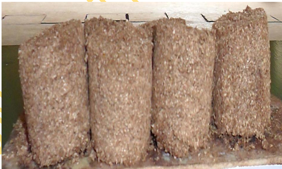
Plate 4.4: Samples of Sawdust Briquettes produced from 1.18mm Particle Size, 20% W / W Binder Concentration at 1.5 MPa
