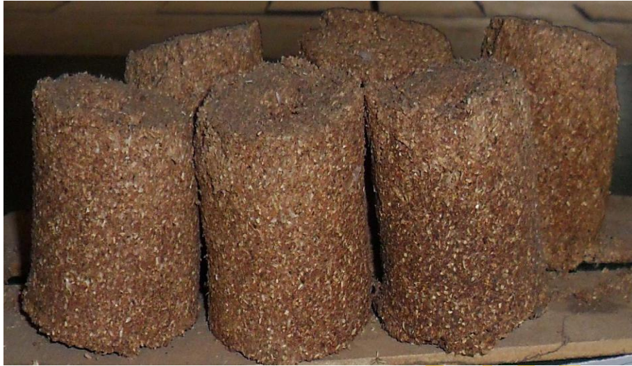
Plate 4.1: Samples of Maize Cob Briquettes produced from 0.6mm Particle Size, 15% w/w Binder Concentration at 1.5 MPa
