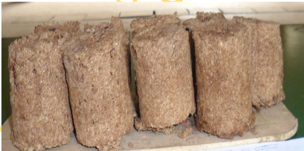
Plate 4.8: Samples of Sawdust Briquettes produced from 1.18mm Particle Size, 25% W / W Binder Concentration at 1.5 MPa
