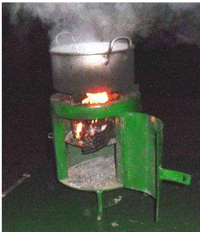
Plate 3.21: Water boiling Test Administered with Briquette Burning Stove at Room Temperature and Pressure
