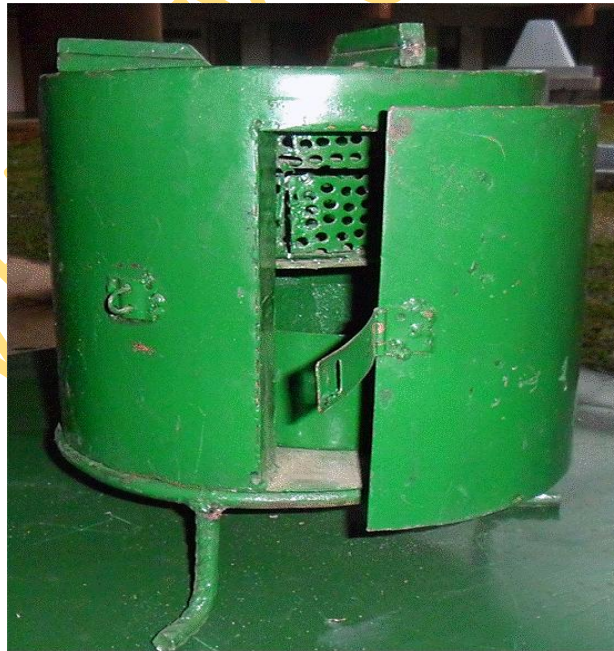
Plate 3.11: Internal Compartment of Briquette Stove
