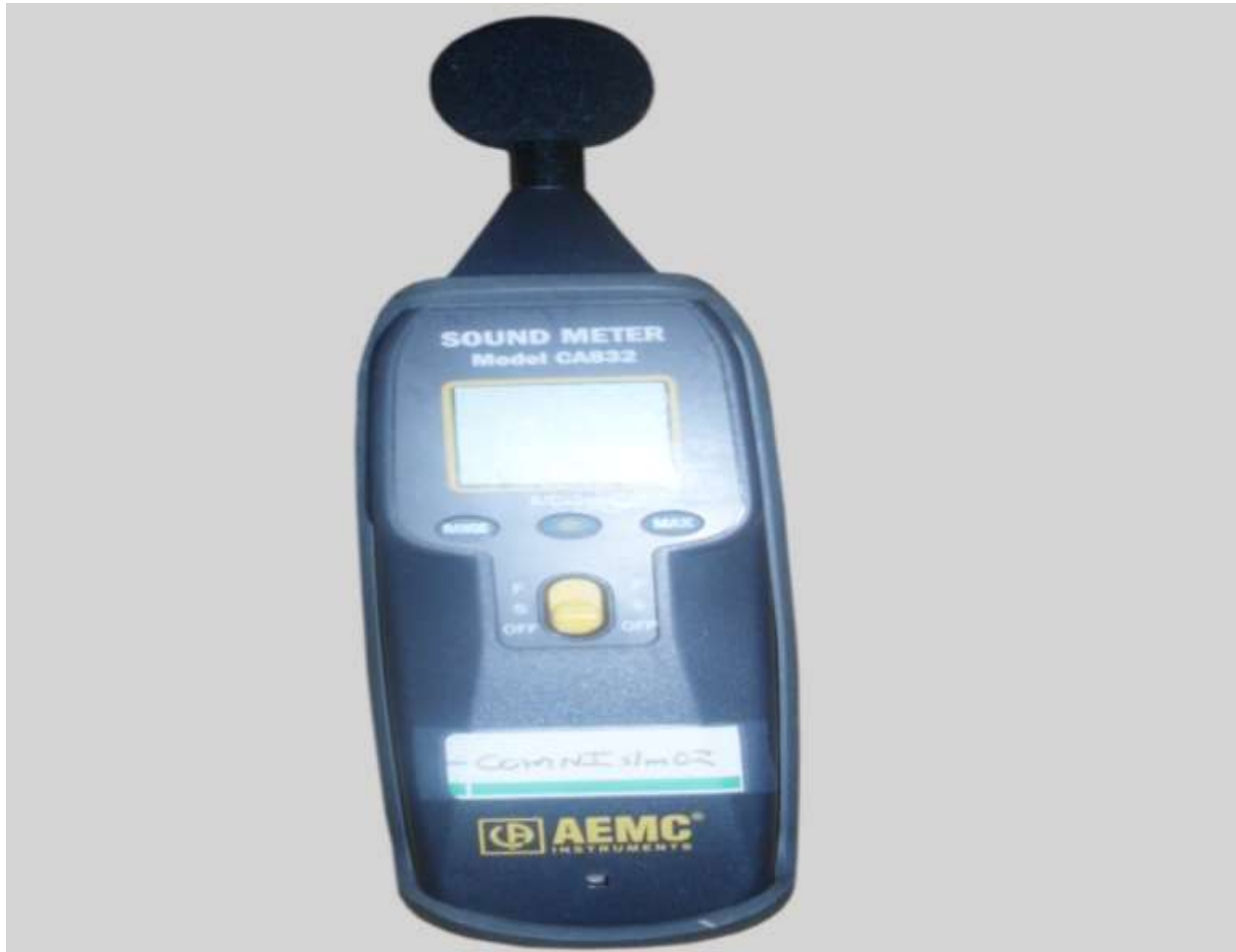
Plate 3.4 Sound level meter
