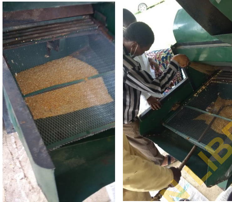
Figure 6: Heaping of grains at cleaning outlet
