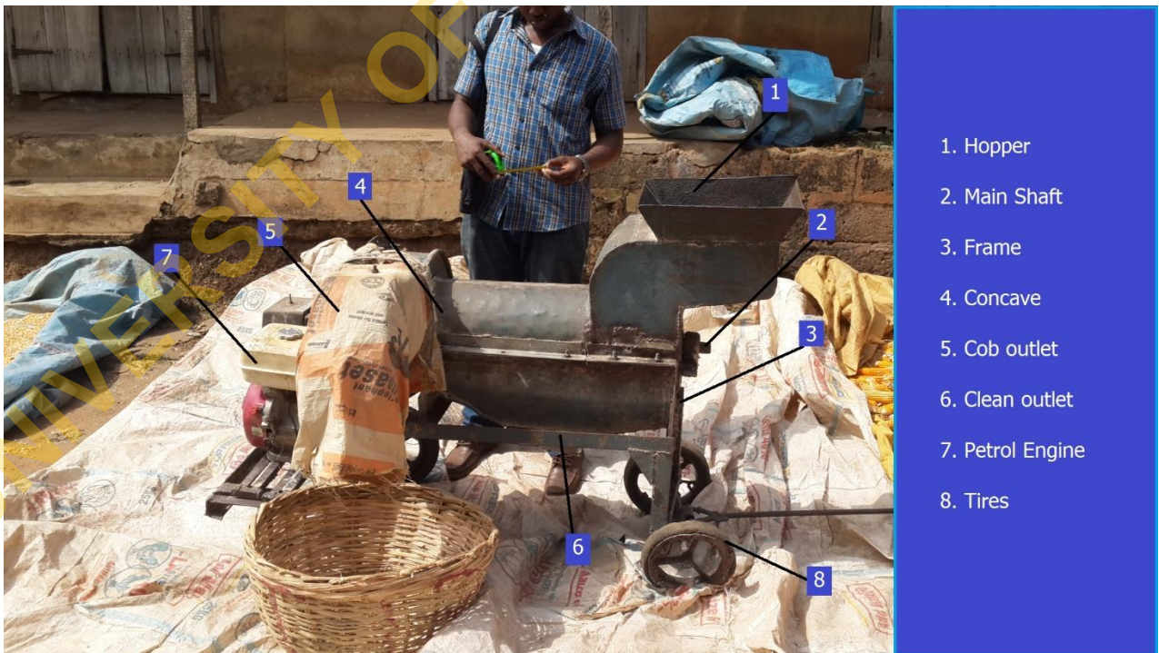
Figure 1. The basic maize sheller typically found in Nigerian markets
