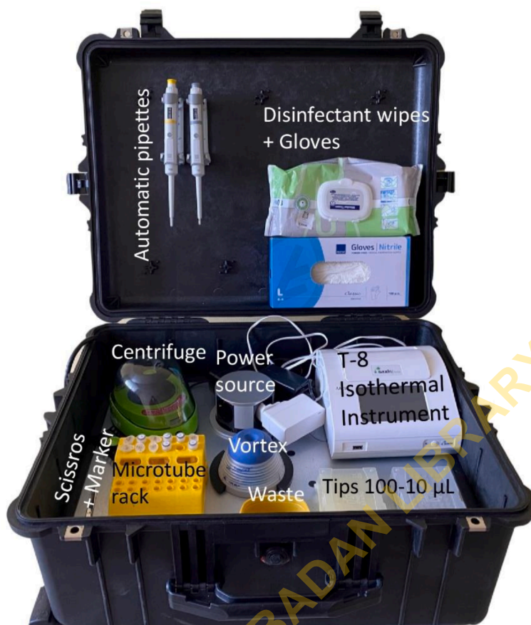
Fig. 3. Example of the suitcase lab, which is fully equipped to perform molecular tests in the field.
