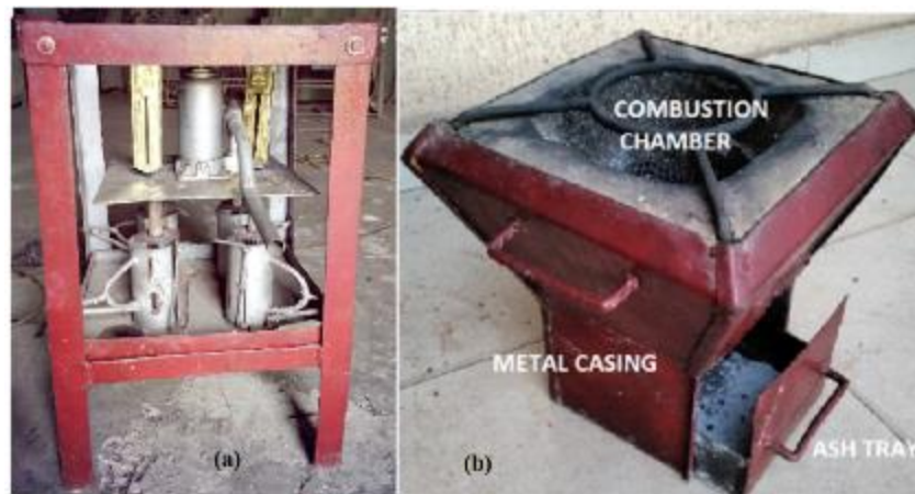
Figure 1. The hydraulic briquetting machine (a) and (b) combustion stove.
