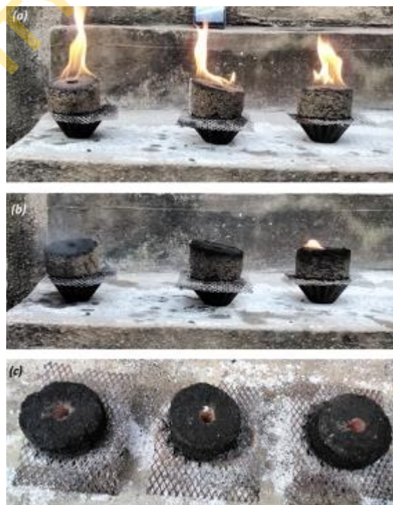
Figure 3. Phase-burning of briquettes in open air [(a) Ignition (b) Flame combustion (c) Char decomposition].
