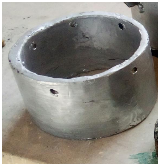
Plate 1.2 Insulated wall of Combustion chamber
