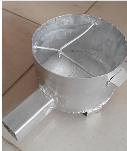
Plate 1.3 Air circulation and Ash Collection pit
