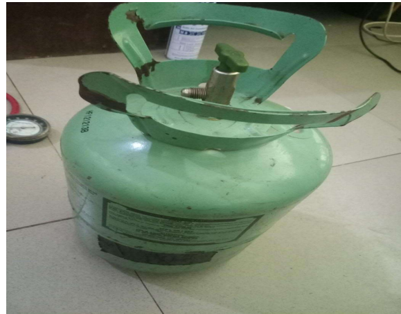
Fig 4: Cylinder containing LPG refrigerant
