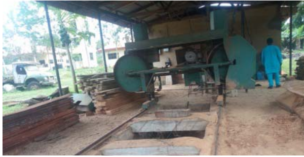
Fig. 1. Locally Fabricated sawmill at University of Ibadan.
