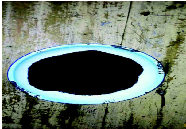
Plate 6: Biochar produced at 400°C and 50 minutes' residence time.
