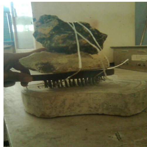
Figure 4. CPB sample under Abrasion resistance testing
