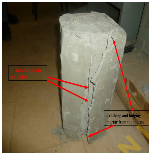
Figure 5. Initial crack, bulging and peeling of mortar.
