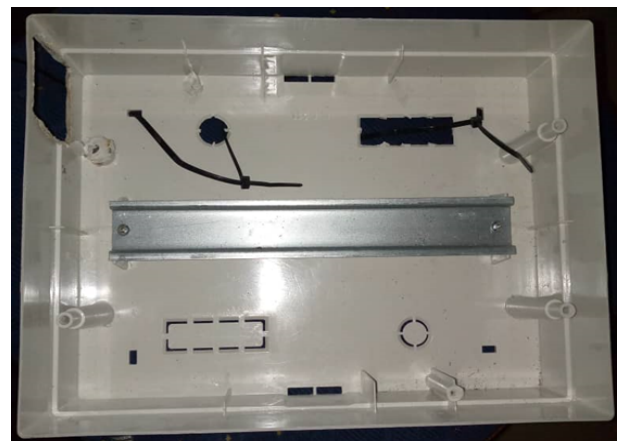
Fig. 3. Inner view of panel box.
