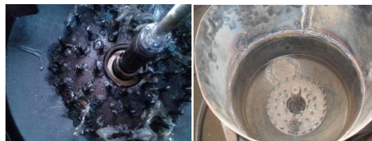
Plate 4 Spike unit in the lacerating chamber
