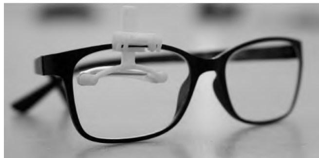
Figure 1: 3D-printed ptosis crutch, described in Saidi, Sivarasu and Douglas, 2018, attached to spectacles.
