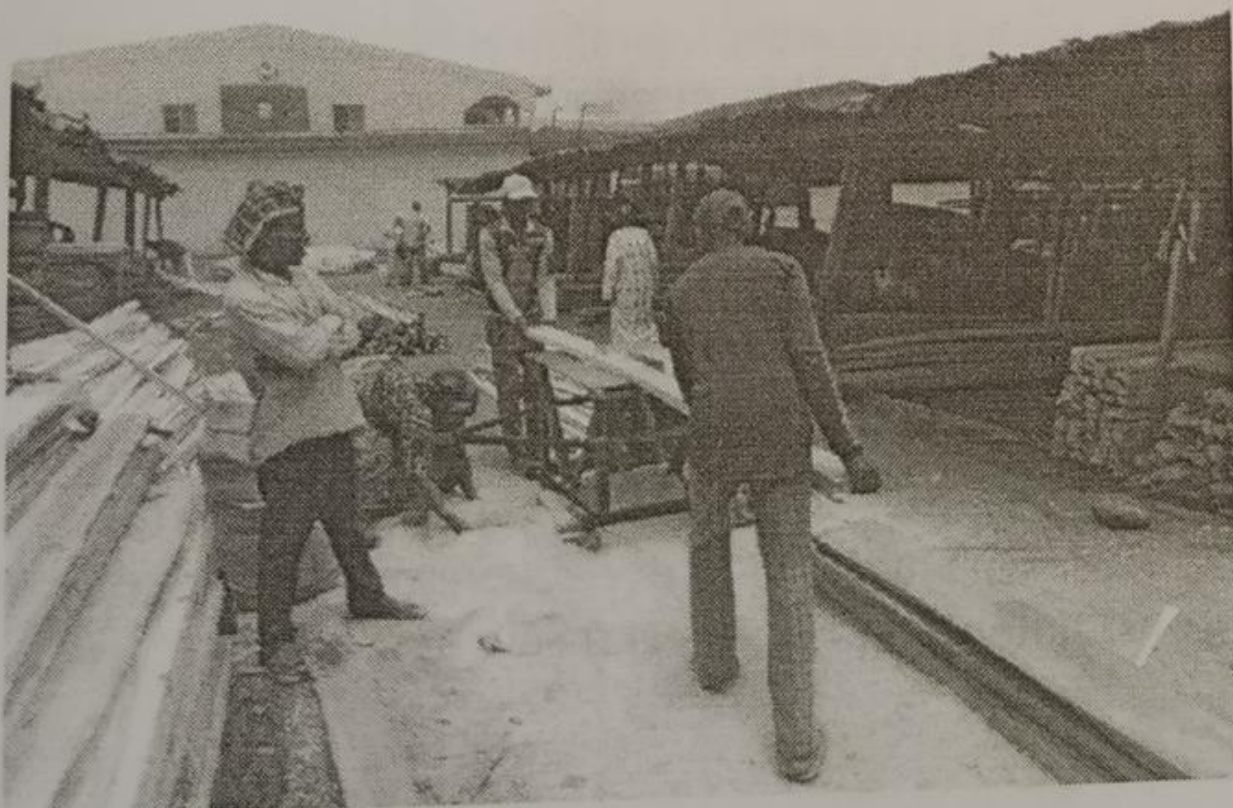
Figure 5: Lumber Reconversion on a Circular saw
