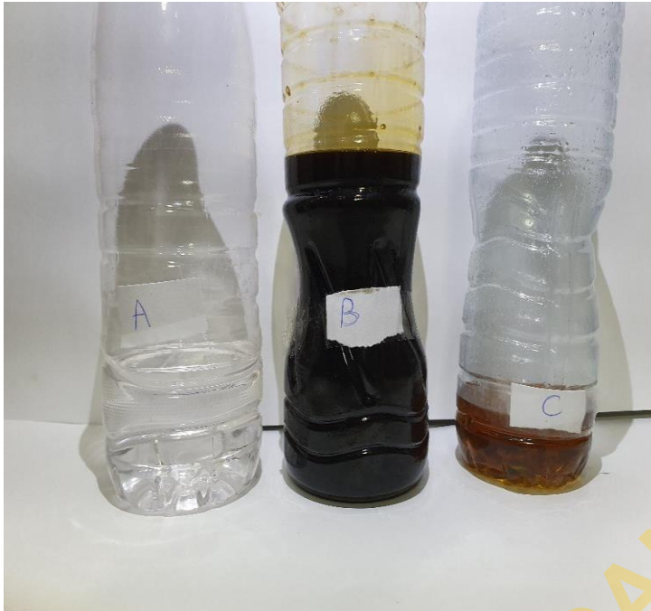
Figure 3.17: Samples of Adulterant (A-Alcohol, B-Used Lubricating Grease, C- Fuel Oil)
