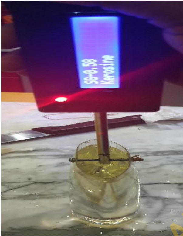
Figure 3.21: Adulterate - meter detecting Impurity in Kerosene.
